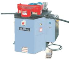
This machine can form radius without pre-bending bars, it comes with a standard 2-speed drive motor.
