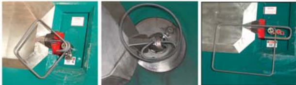
MINFORM 616 Pictured above. Below examples of stirrups produced on the 616.
