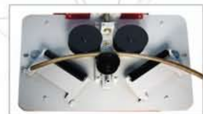
One step radius bending process
